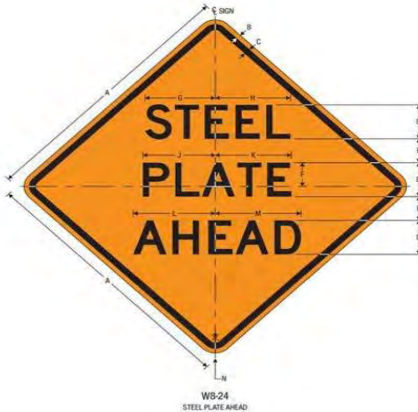
FIGURE 9-10. STEEL PLATE AHEAD SIGN DETAIL
