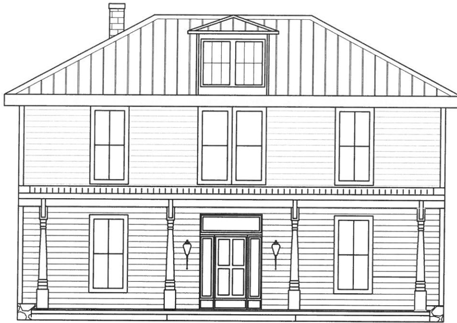
PROPOSED FRONT ELEVATION WITH SINGLE CHIMNEY OPT. #1 DOOR WITH SIDE LIGHTS SCALE: 1/8" = 1'-0"
