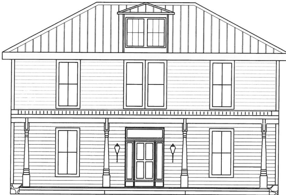
PROPOSED FRONT ELEVATION WITHOUT CHIMNEYS OPT. #1 DOOR WITH SIDE LIGHTS SCALE: 1/8" = 1'-0"
