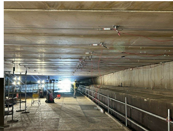
Bridge Weight Testing
