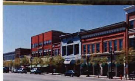
Example: Express façade components using methods that will help convey a human scale. Comparable to this historic building wall, dividing a single development into distinct façade modules is one example of how to accomplish this.
