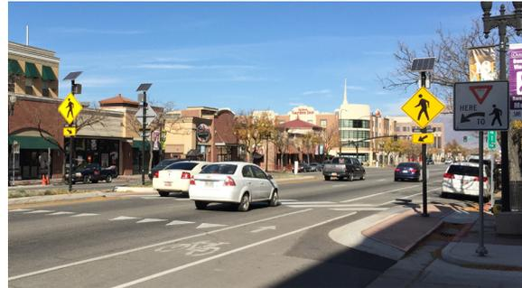
Figure 4.13 Rapid Rectangular Flashing Beacons in Ogden, UT
