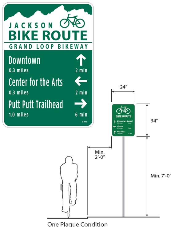
Figure 4.20 Typical Bikeway Wayfinding Signage
