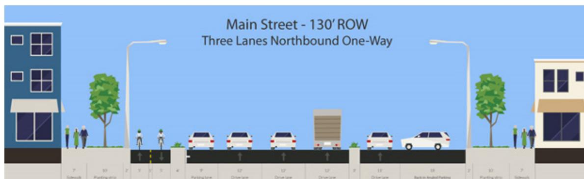
Figure 4.24 Possible Main St. Couplet-scenario cross-section
