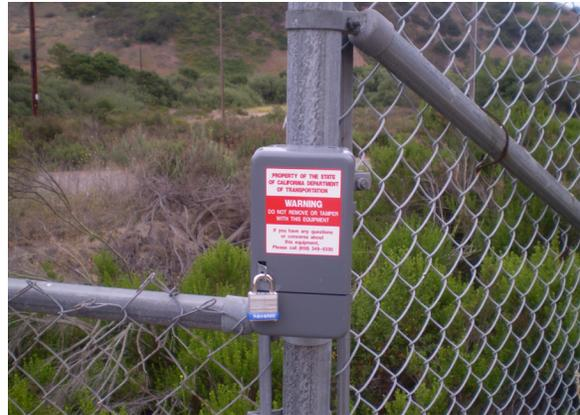
Figure 4.23 Infrared Trail User Counter
