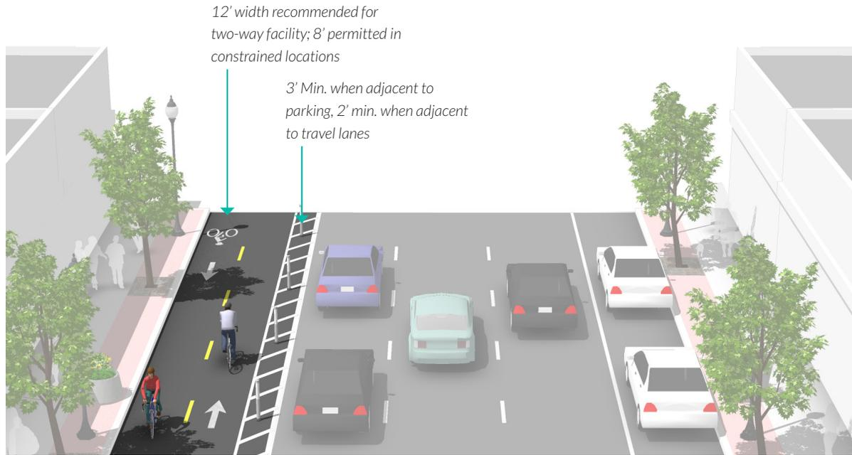
Figure 4.8 Typical Two-way Protected Bike Lane
