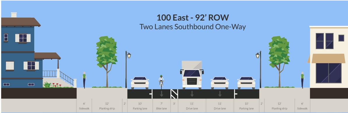
**Figure 4.26 Possible 100 East Couplet-scenario cross-section**
