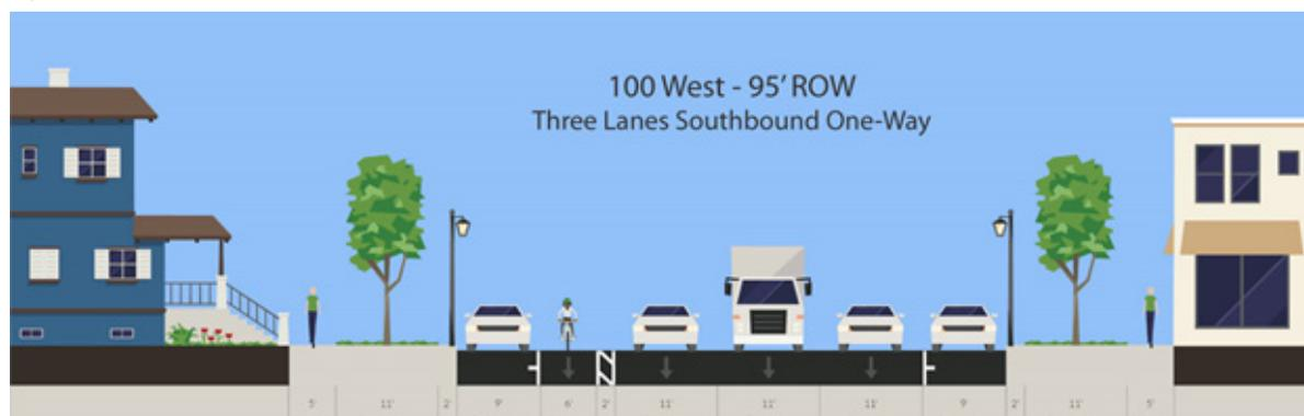
Figure 4.25 Possible 100 West Couplet-scenario cross-section
