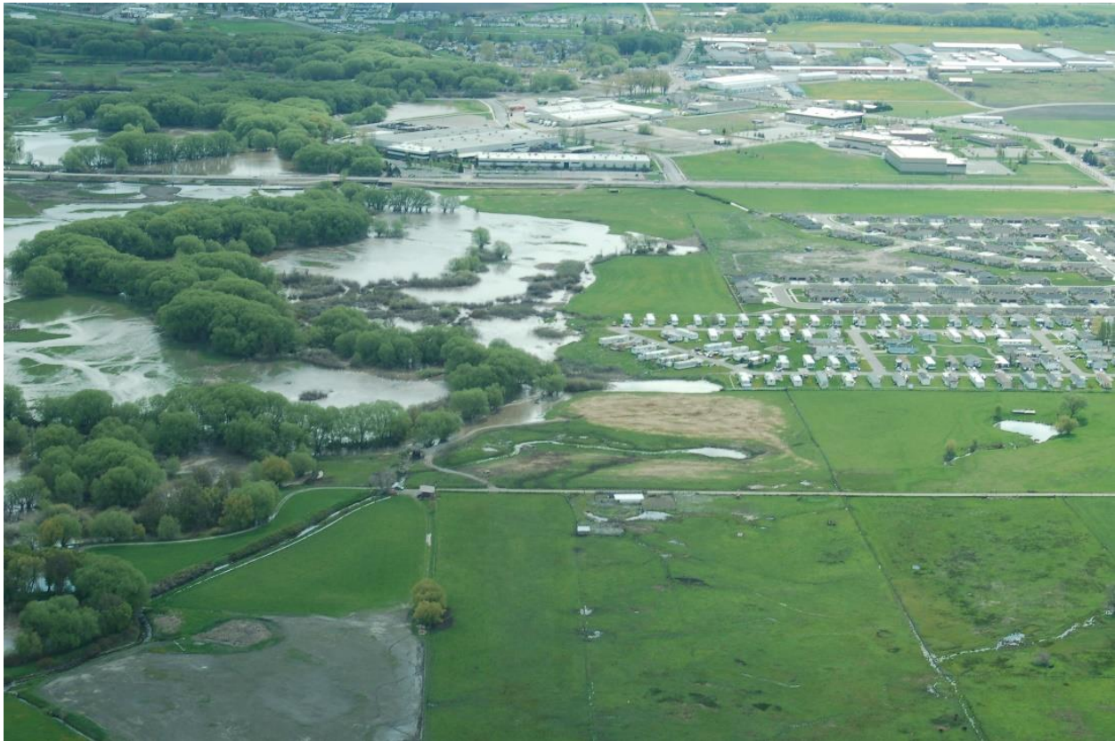
Figure 1: The Logan River Golf Course (upper right) and Rendezvous Park flooded during a storm in 2011. The park and the golf course provided open space for the river to overflow, which reduced the flood risk to neighboring communities. Photo courtesy of Civil Air Patrol
