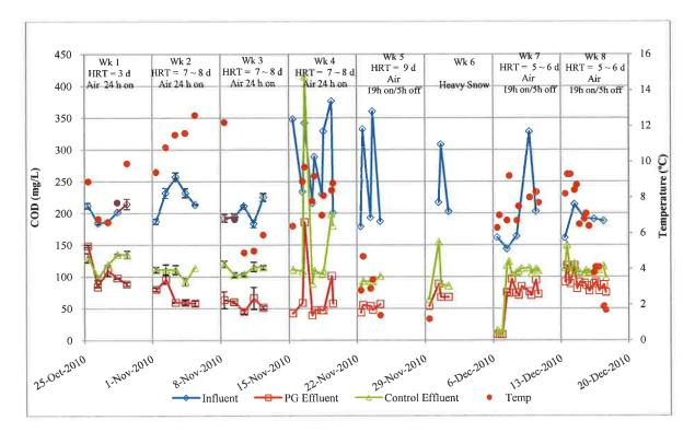
Figure 4: Week 1- 8 of oxygen demand results, measured as COD.
