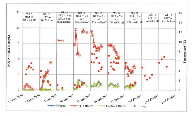
Figure 15: Week 9 - 17 of NO<sub>3</sub><sup>-</sup>/NO<sub>2</sub><sup>-</sup> results.
