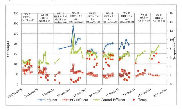
Figure 5: Week 9 - 17 of oxygen demand results, measured as COD. Wastewater Compliance Systems, Inc Proprietary Information ©2011
