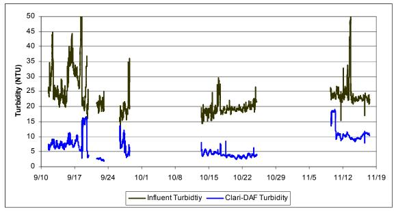
Figure 5. Raw Water and Clari-DAF System Effluent Turbidity. \*
