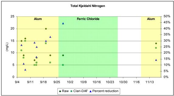
Figure 10. Raw Water and Clari-DAF System Effluent Total Kjeldahl Nitrogen.
