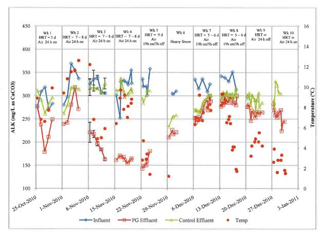
Figure 19: Week 1- 10 of Alkalinity results. ALK tests were discontinued after week 10. Wastewater Compliance Systems, Inc Proprietary Information ©2011
