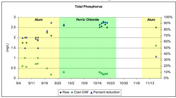
Figure 9. Raw Water and Clari-DAF System Effluent Total Phosphorus.
