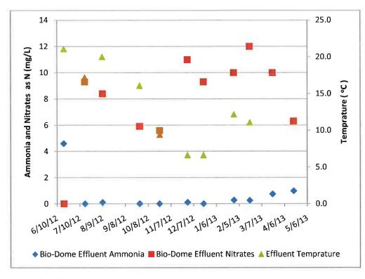
Figure 21 – Comparison of Ammonia and Nitrate in Effluent as a Result of Air Cycling Initiated at the End of March 2013 at Quincy, CA
