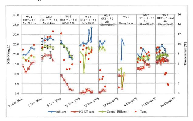
from 2 to 3 to 4 hours per day. The stair-step effect on the ammonia concentrations in the PG Tank effluent is apparent.
