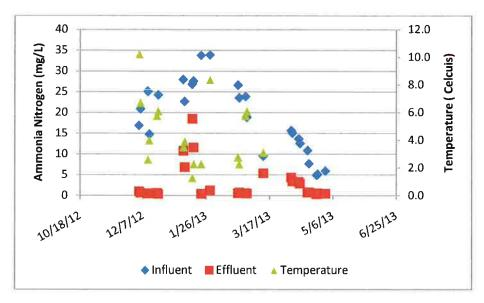
Figure 13 - Concentrations In and Out of the Pilot Unit at West Branch, Iowa
