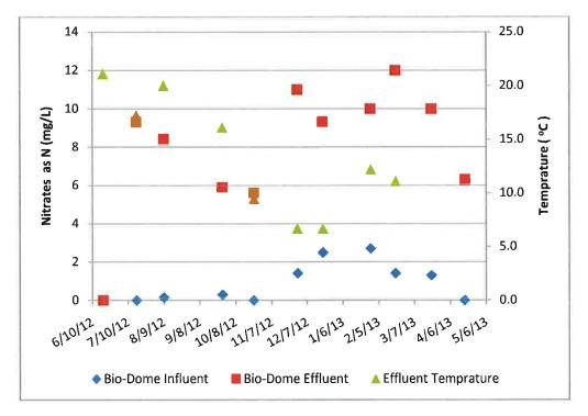
Figure 20 - Concentrations of Nitrate In and Out of the Pilot Unit at Quincy, CA
