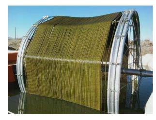
Rotating Algal Biofilm Reactor (RABR) designed by SWBEC is currently being tested at the Logan lagoon facility.
