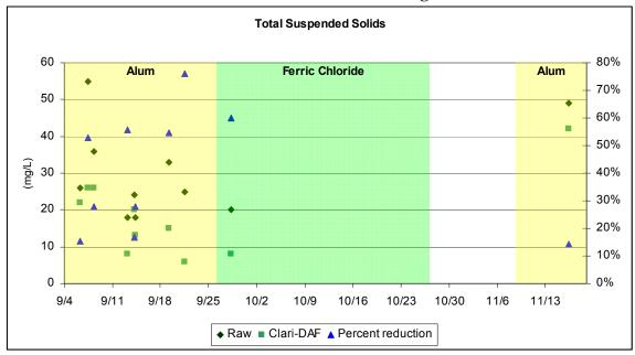
Figure 11. Raw Water and Clari-DAF System Effluent Total Suspended Solids.
