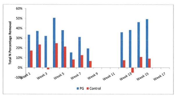
Figure 18: Total Nitrogen percentage removal from influent to effluent, PG vs. Control. Wastewater Compliance Systems, Inc Proprietary Information ©2011
