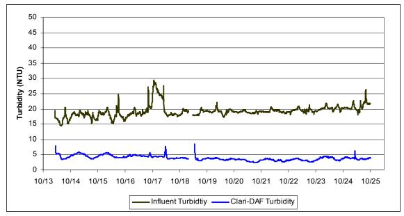
Figure 7. Raw Water and Clari-DAF System Effluent Turbidity Ferric Chloride 4 gpm/ft<sup>2</sup> 10/13-25/2011. \*
