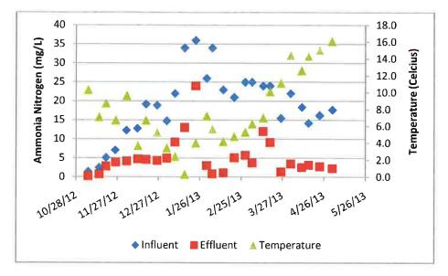
Figure 16 - Concentrations In and Out of the Pilot Unit at Naturita, CO
