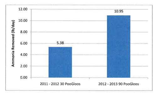
Figure 22 - Cell 2 Removal of Ammonia N, Year on Year Comparison, Jackpot, NV
