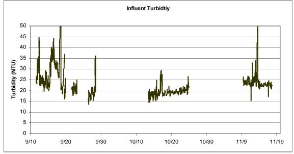
Figure 2. Raw Water Turbidity During the Pilot Study. \*
