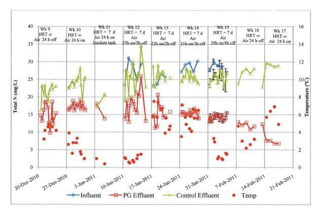
Figure 17: Week 9 - 17 of Total Nitrogen results. Note in weeks 13 to 15 evidence of improved N removal by Poo-Goos due to air cycling.
