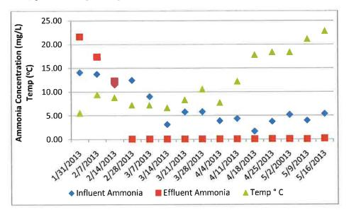
Figure 15 - Concentrations In and Out of the Pilot Unit at Laddonia, MO
