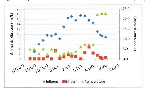
Figure 11 - Concentrations In and Out of the Pilot Unit at Lenox Iowa
