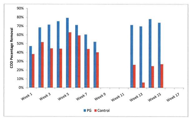
Figure 6: COD percentage removal from influent to effluent, PG vs. Control.
