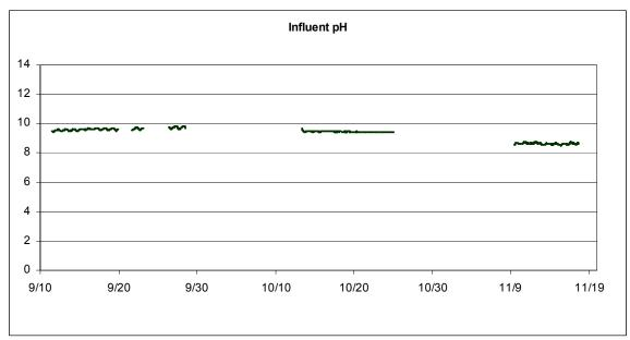
Figure 3. Raw Water pH During the Pilot Study. \*
