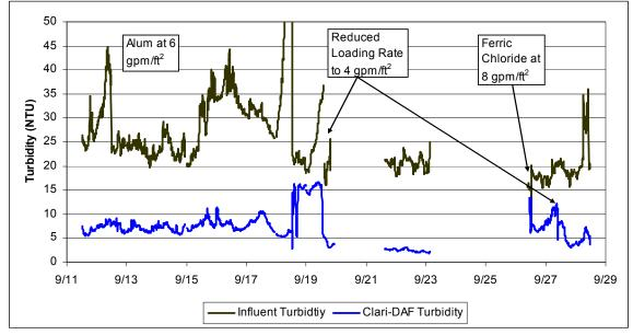
Figure 6. Raw Water and Clari-DAF System Effluent Turbidity 9/11-29/2011. \*
