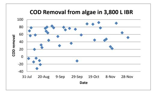
Figure 2. Chemical oxygen demand removal from algae fed to the 3,800 l IBR during the time period August through November, 2011.
