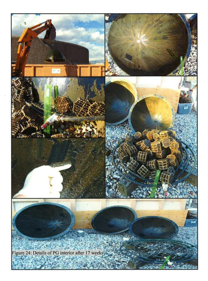
Following week 17, one PG was removed from the mid-point of the PG Test tank and taken apart. Biofilm samples were taken from 9 locations inside the domes. The results show that the dry mass of the biofilm covers a colonized surface at 34.6 g/m<sup>2</sup> and the amount of P in the dry mass is 1.4%.
