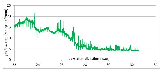
Fig 1 Biogas production at days 22 -33 in the 60 I IBR. The HRT when this data was taken was24 days).
