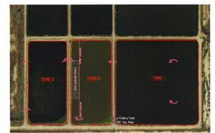
Figure 5 -Layout of sampling locations at Plain City wastewater lagoon
