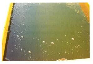
Figure 29: Close up of Control tank at point farthest from influent around week 16. Note turbidity and absence of filamentous algae.
