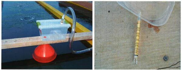
Figure 10: Measurement of volatized ammonia in off-gas. Red funnel test apparatus and close-up of yellow test tube are shown after exposure to escaping air bubbles for 3 weeks to test for the presence of volatized ammonia. Yellow granules would turn purple in the presence of ammonia.
