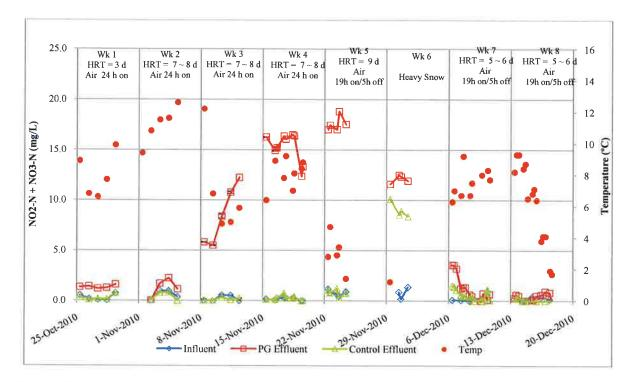
Figure 14: Week 1 - 8 of NO<sub>3</sub><sup>-</sup>/NO<sub>2</sub><sup>-</sup> results.
