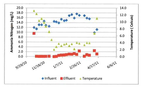
Figure 9 - Concentrations In and Out of the Pilot Unit at Gresham, WI
