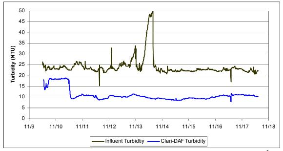
Figure 8. Raw Water and Clari-DAF System Effluent Turbidity Alum 4 gpm/ft<sup>2</sup> 11/9-17/2011. \*
