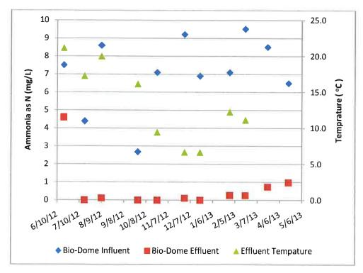
Figure 19 - Concentrations of Ammonia In and Out of the Pilot Unit at Quincy, CA
