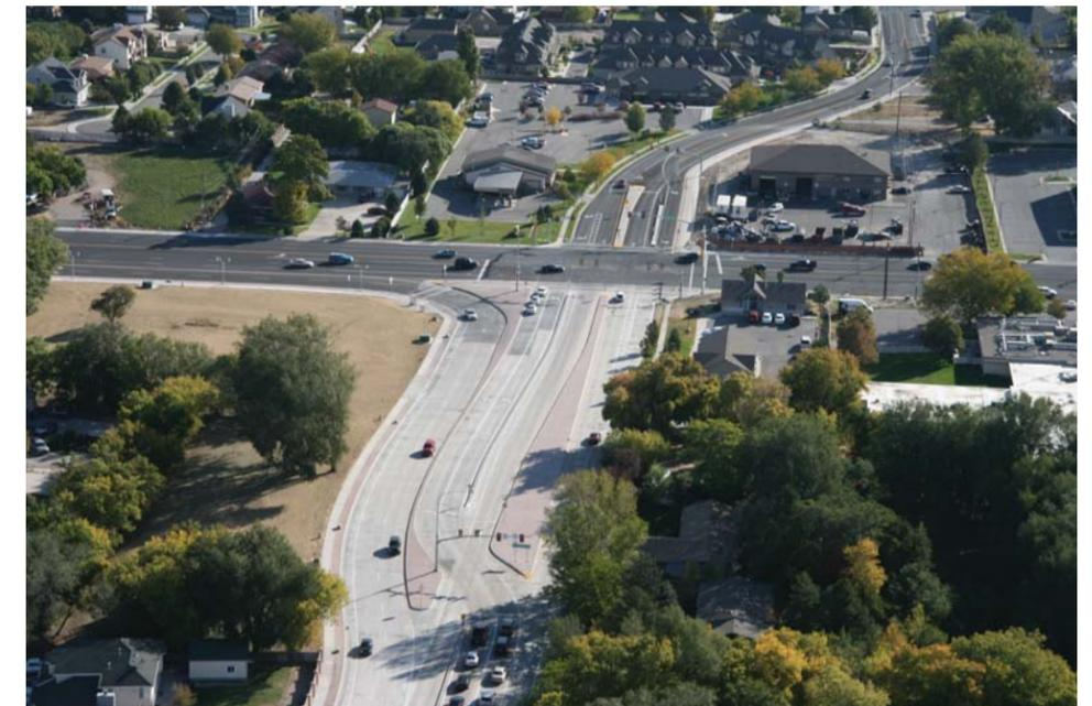
Figure 2-18 Continuous Flow Intersection
