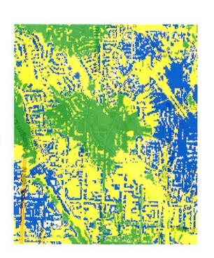
**Coverage** is best shown via coverage maps. RF engineers use tools that take into account terrain, vegetation, building types, and WCF specifics to model the existing coverage and predict what we expect to see with the addition of a proposed WCF.
