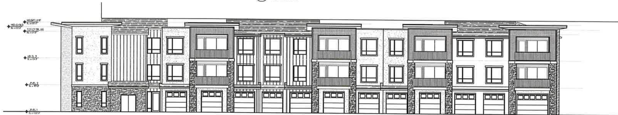
3 50-UNIT APARTMENTS SOUTH ELEVATION SCALE: 1/8"=1'-0"
