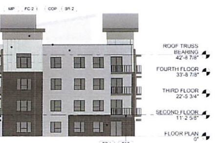
3 BLDG 3 WEST EXTERIOR ELEVATION 1/16" = 1'-0"
