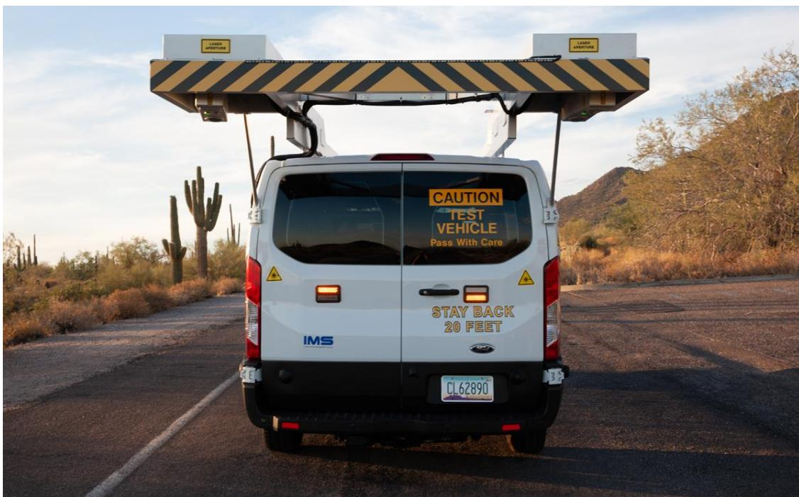
**Figure 10 - LCMS2 data collection vehicle**
