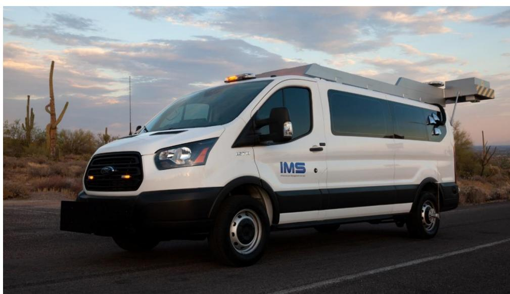
**Figure 1 - IMS Road Surface Tester (RST)**
