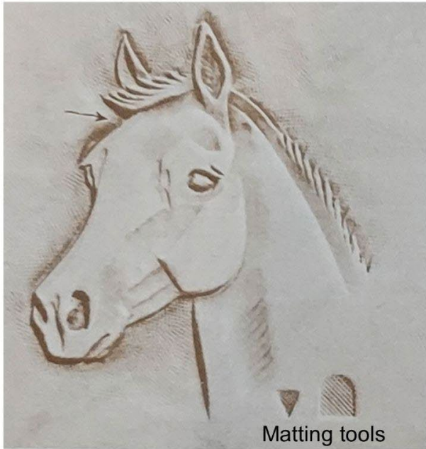
The arrow shows use of pointed matting tool. Matt background with larger matting tool and hard to get places with smaller.
