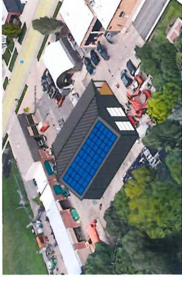
Image 2: DPW, Roof Mounted, 20 kw Solar Array
