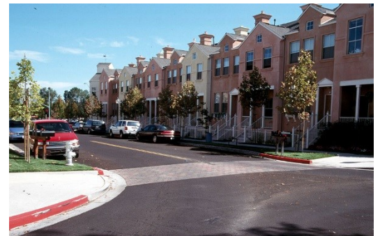
This marked pedestrian crossing (above) uses paint and different paving materials to alert motorists to areas where pedestrians may be present.
