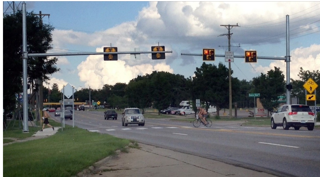
Example of Pedestrian Crossing on Orchard Lake Road in Keego Harbor. This light only changes when activated by a pedestrian or cyclist.
