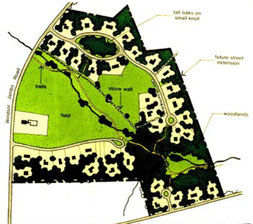
Figure D-5. This figure illustrates how reorganizing the subdivision creates community accessible, preserved open space.
