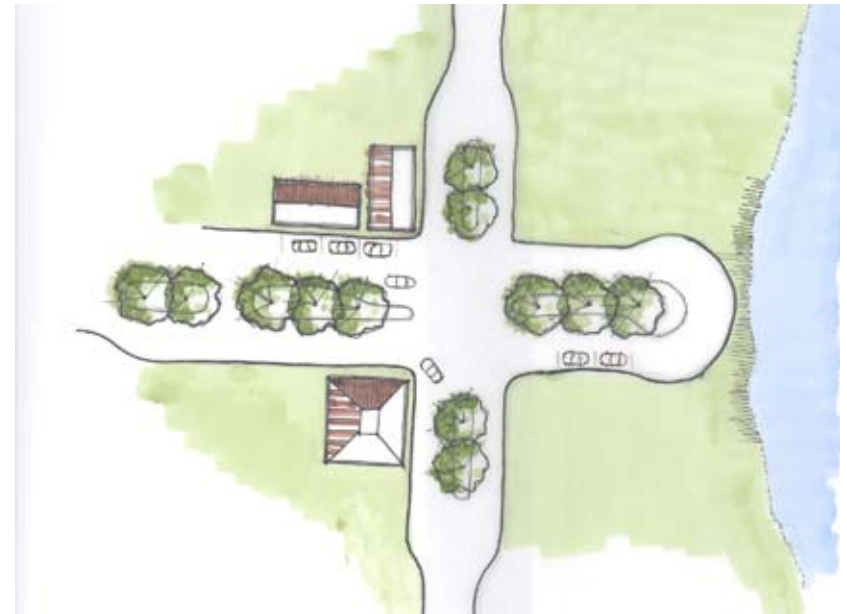
Figure 34. Bayview Avenue could be widened to improve circulation and allow on-street parking.
