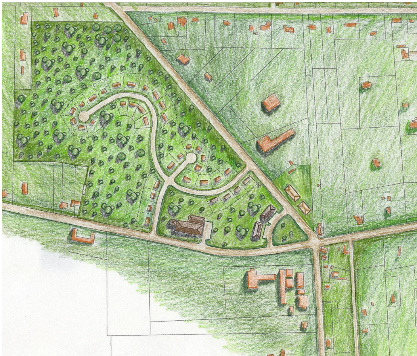
Figure 27. Scenario 2: Same number of houses as in Scenario 1, clustered on a smaller portion of the site. The lot sizes are one-half acre on average.
