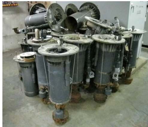
These grinder pumps were all damaged during Hurricane Irene and were replaced by the Department of Public Works.
