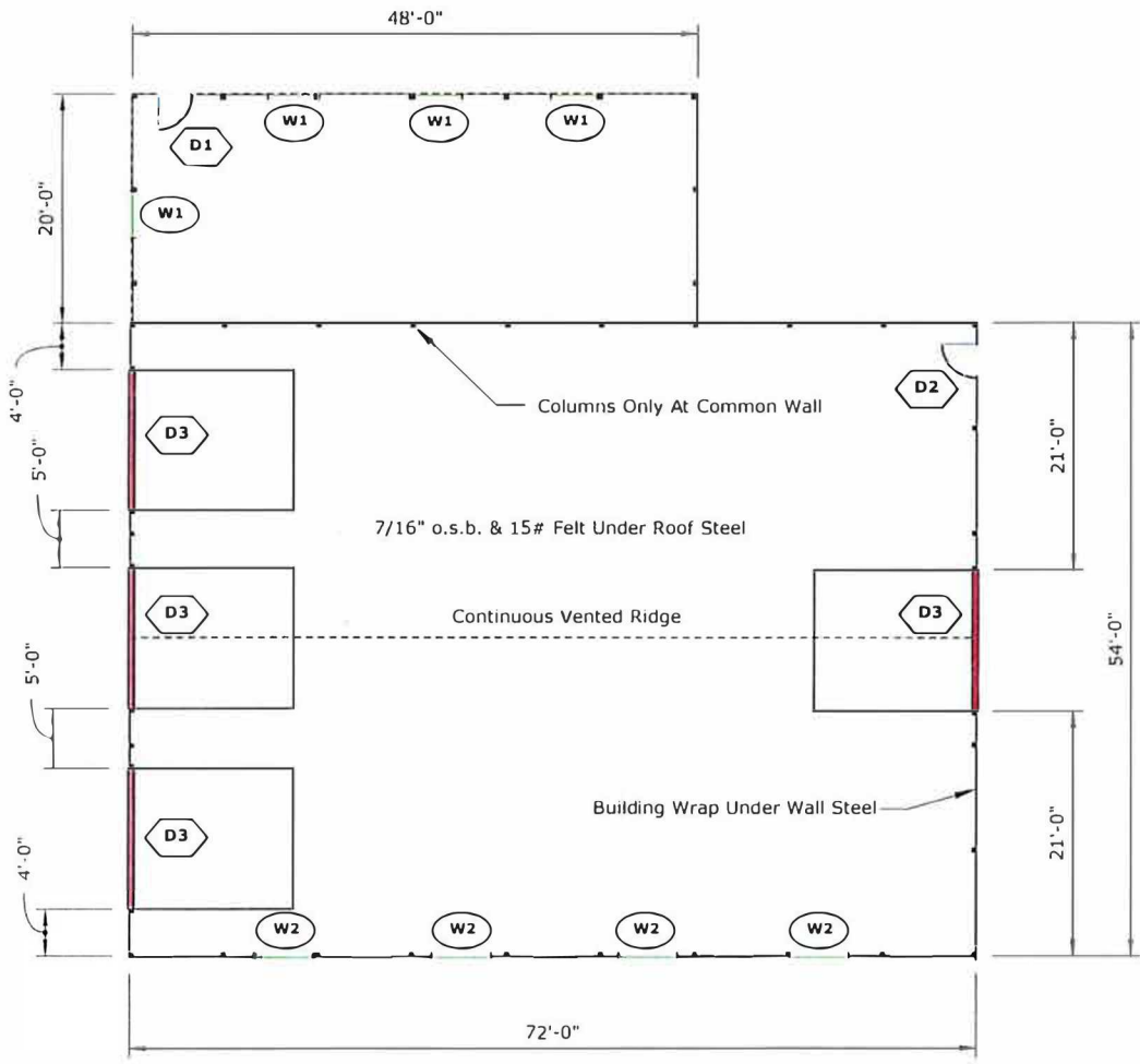
FLOOR PLAN FBI Building 54' x 72' x 16' I.C. w/20' x 48' x 10' Lean-To Office Sidewall Columns & Trusses Space at 8' O.C. Designed for 30 psf Ground Snow Load
