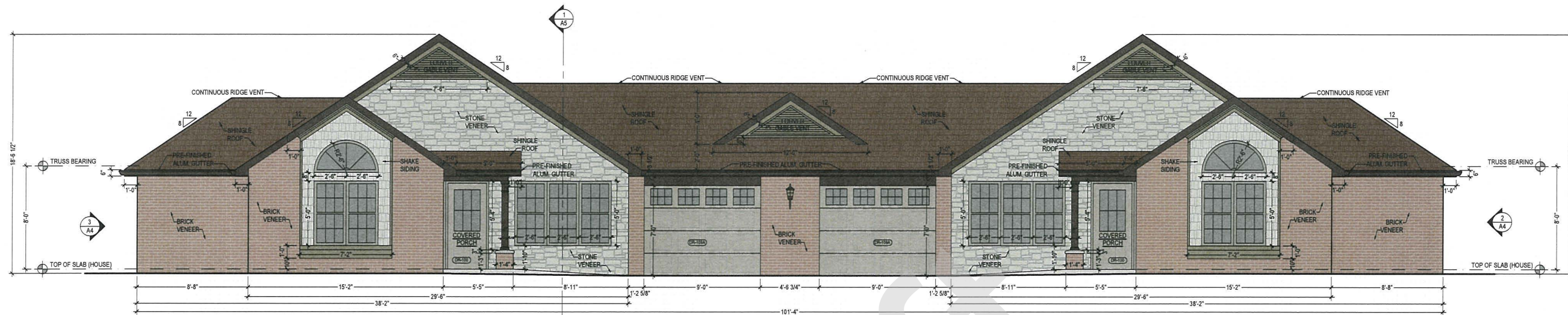
1 FRONT ELEVATION - BUILDING TYPE-C SCALE: 1/4" = 1'-0"
