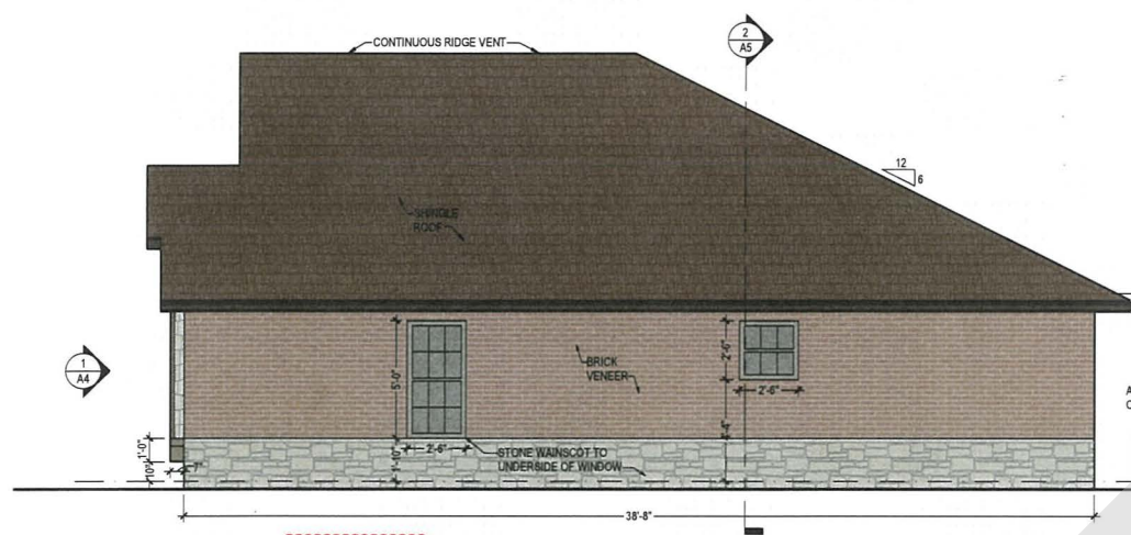
2 SIDE-1 ELEVATION - BUILDING TYPE-B SCALE: 1/4" = 1'-0"
