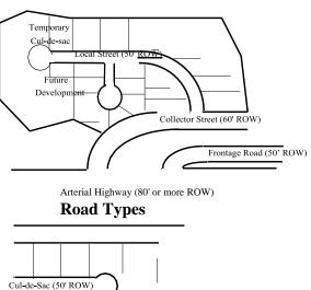
(2) <u>Minor/Residential</u> streets not classified in a higher system, primarily providing direct access to abutting land and to collector streets
