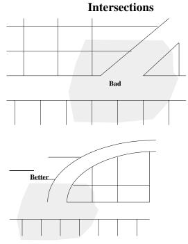
intersection. Where roads and streets intersect arterial or collector routes, their alignment will be continuous. Intersections of arterial or collector roads and streets will be at least 800 feet apart.
