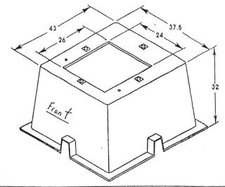
2) FOR ALL THREE PHASE PAO MOUNTED TRANSFORMERS SHALL USE A CONCRETE VAULT.
