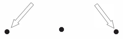
Bollards are to be place 2 feet from side of concrete vault.
