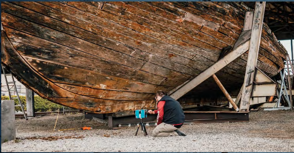
Above: A Texas A&M student uses LIDAR to document the Equator.
