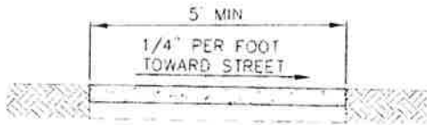
4" CONCRETE SIDEWALK (3500 psi @ 28 DAYS)
