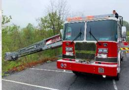
KME's platform has an elevation range that allows you to go -12° below horizontal without any impact on platform capacity and while flowing 2000 GPM water.
