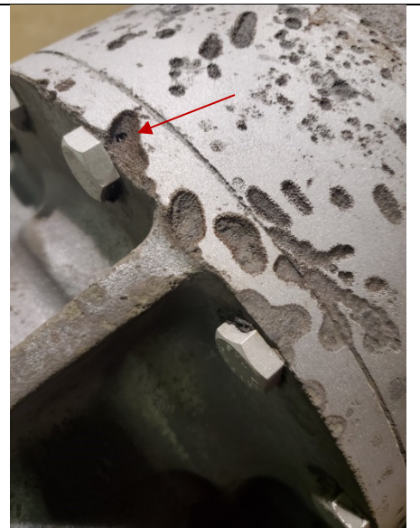
Pitting completely through to threaded S.S. Bolts
