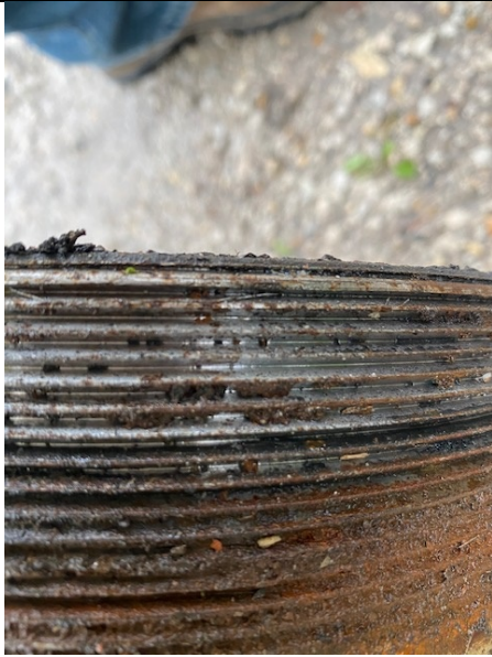
Rolled & flattened leading edges of threads
