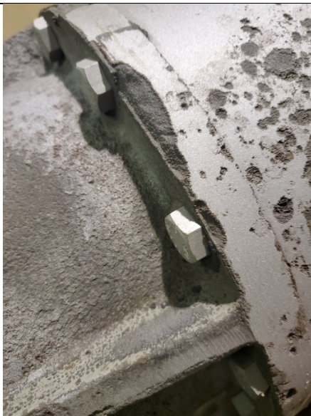
OD of bowl assembly with pitting
