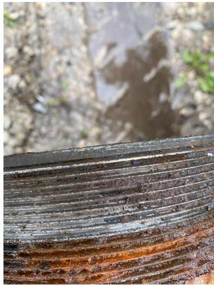
Rolled & flattened leading edges of threads
