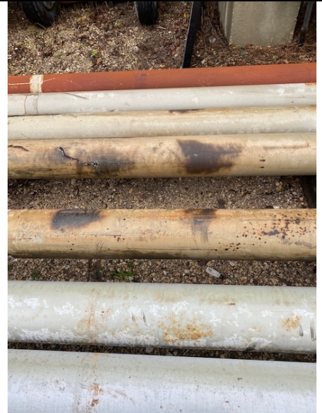
OD of epoxy coating on 8" column pipe deterioration
