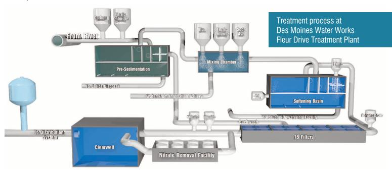
Throughout the treatment process, DMWW's laboratory staff performs 100-150 tests each day to ensure the highest quality water is produced. An additional series of 50-60 daily tests on the untreated water sources allows laboratory staff to identify any necessary changes needed in the treatment process before the water enters the treatment plants.
