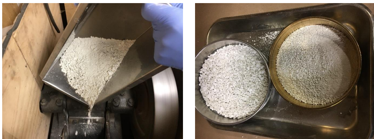
Figure 2. Typical CaO, as prepared for slaking, involves rapid crushing to -6 mesh, screening, and riffing to obtain a representative sample.
