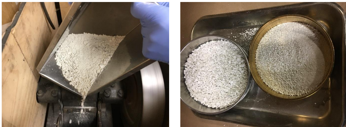
Figure 2. Typical CaO, as prepared for slaking, involves rapid crushing to -6 mesh, screening, and riffling to obtain a representative sample.
