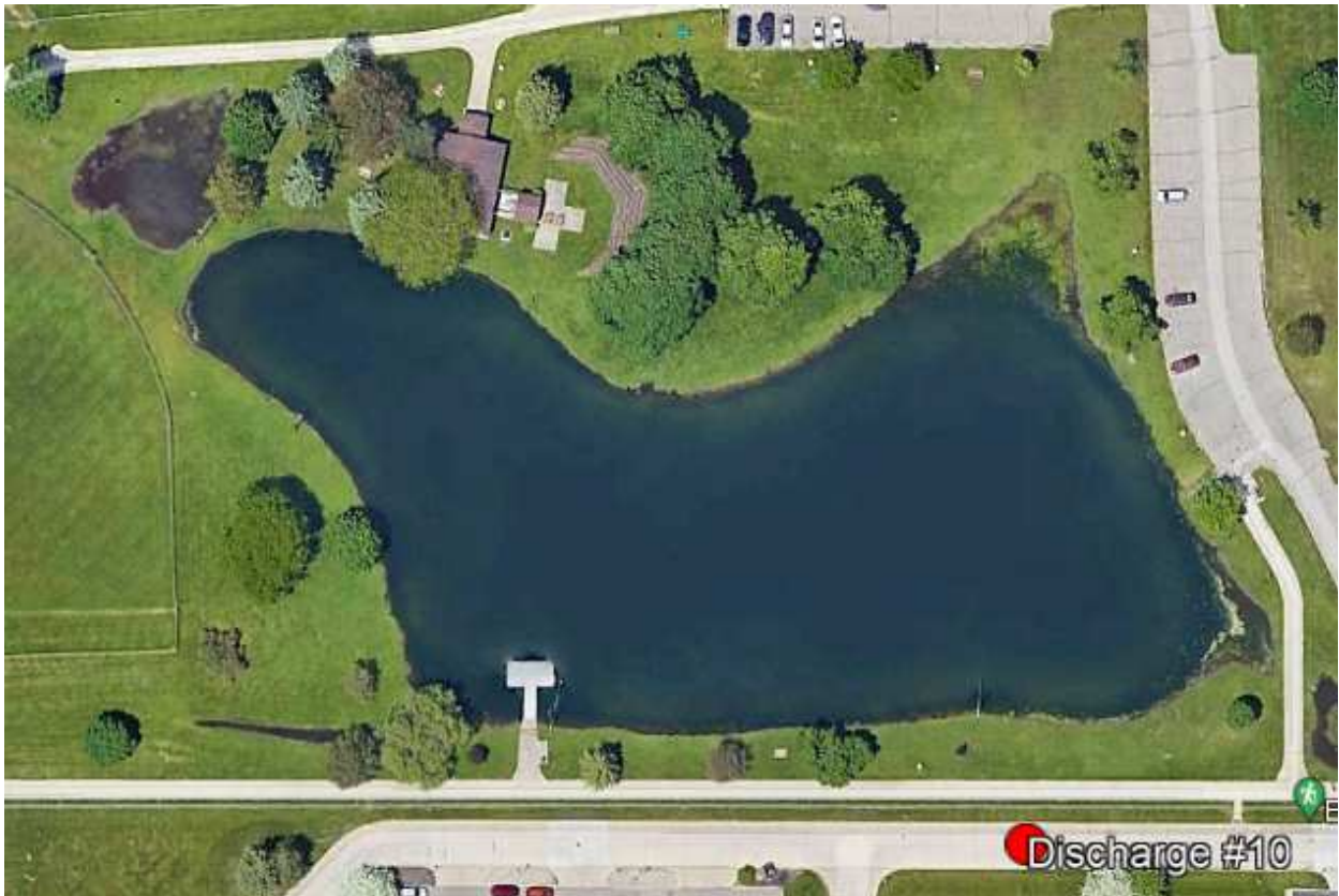
Figure 3 - Pond located at Sharp Park. Flow leaves the pond on the south side to the storm sewer system.
