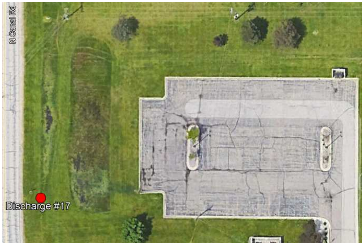
Figure 4 - General site view. Discharge location is at the red dot, however there is a ponding area and swale.
