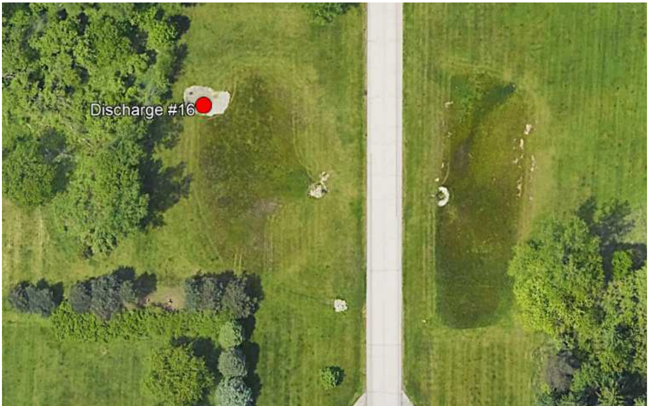
Figure 6 - Aerial view of detention system. Where the red dot is located is the discharge location from the system.
