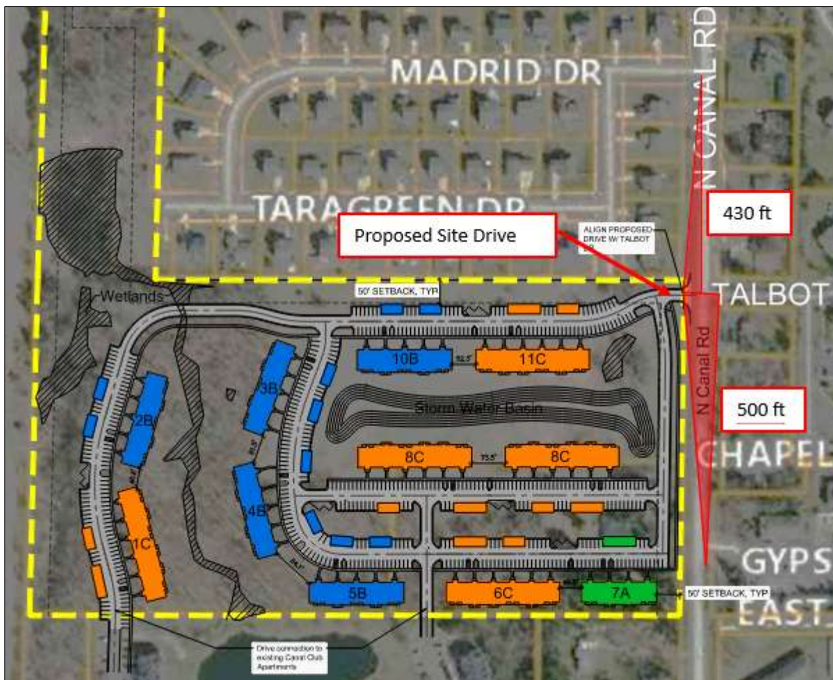
EXHIBIT 14: SIGHT DISTANCE TRIANGLE AT CANAL RD AND SITE DRIVEWAY
