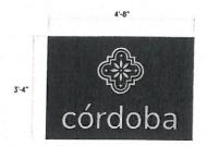
High Density Urethane panel logo to be routed into surface and paint filled
