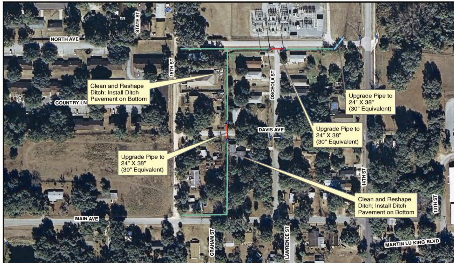
Figure 10-5 Basin 1W, Area 1B Proposed Osceola Street Ditch Improvements
