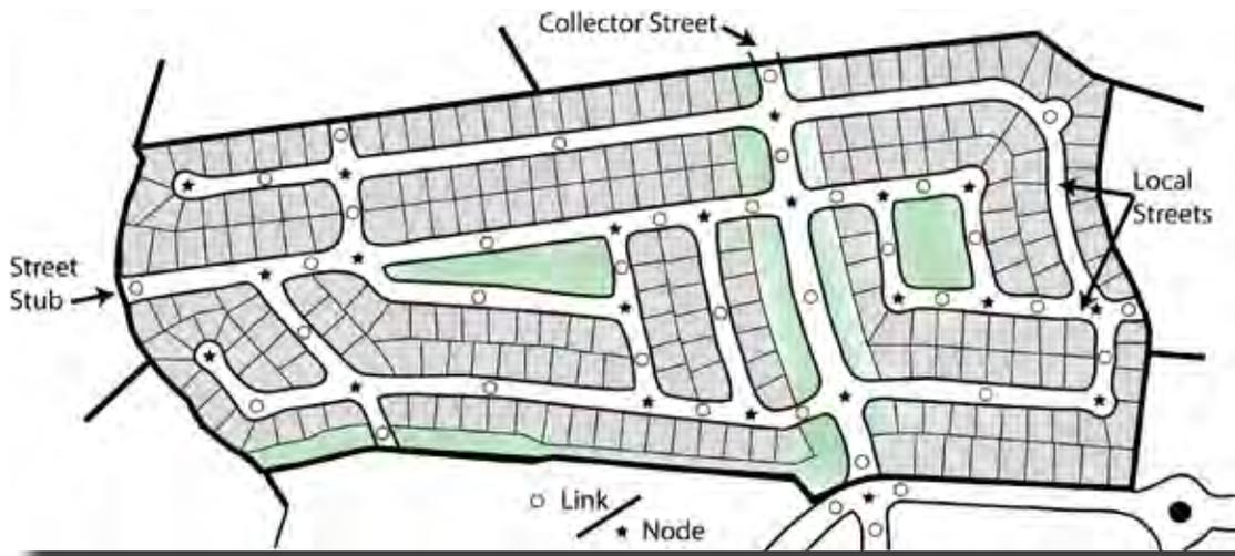
This diagram illustrates how a suburban subdivision can be designed and evaluated for connectivity. The Virginia Department of Transportation has recently established new guidelines for connectivity to accept secondary roads into the state system. Additionally, connectivity provides alternative routes to relieve congestion on primary roads and improves access and response times for emergency response vehicles.
