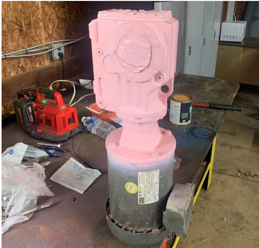
Repair and painting of drive for 12 MGD screen at the WPCF headworks (February 2021)
