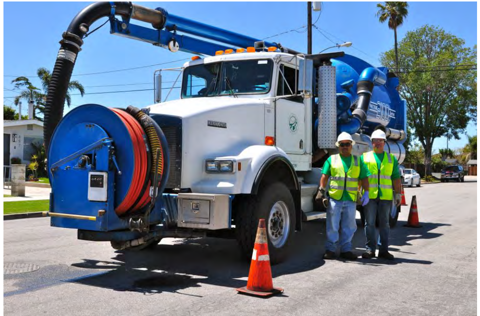
1992 Sewer Combination Cleaning Truck and CMSD WMWs
