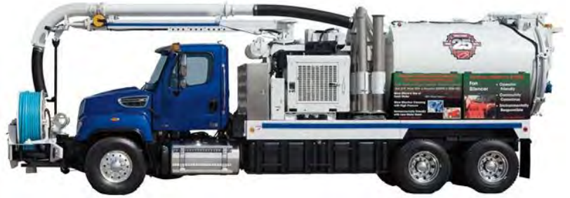
Sewer Combination Cleaning Truck
