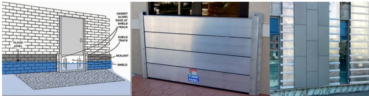
Figure 8: Floodproofing conceptual design
