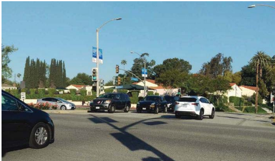
Figure 3: A long queue of southbound vehicles blocked northbound vehicles from completing left turns at Granada Avenue/Huntington Drive. Vehicles unable to complete their movement within one phase waited in the middle of the intersection until traffic cleared.
