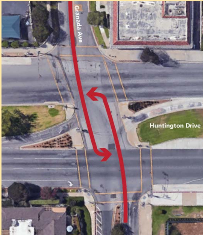
Existing issues: North-south left turn paths interlock at Huntington Drive and Granada Avenue
