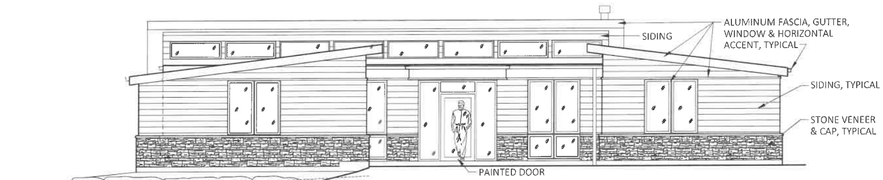
PROPOSED EAST ELEVATION Scale: 1/8" = 1'-0"
