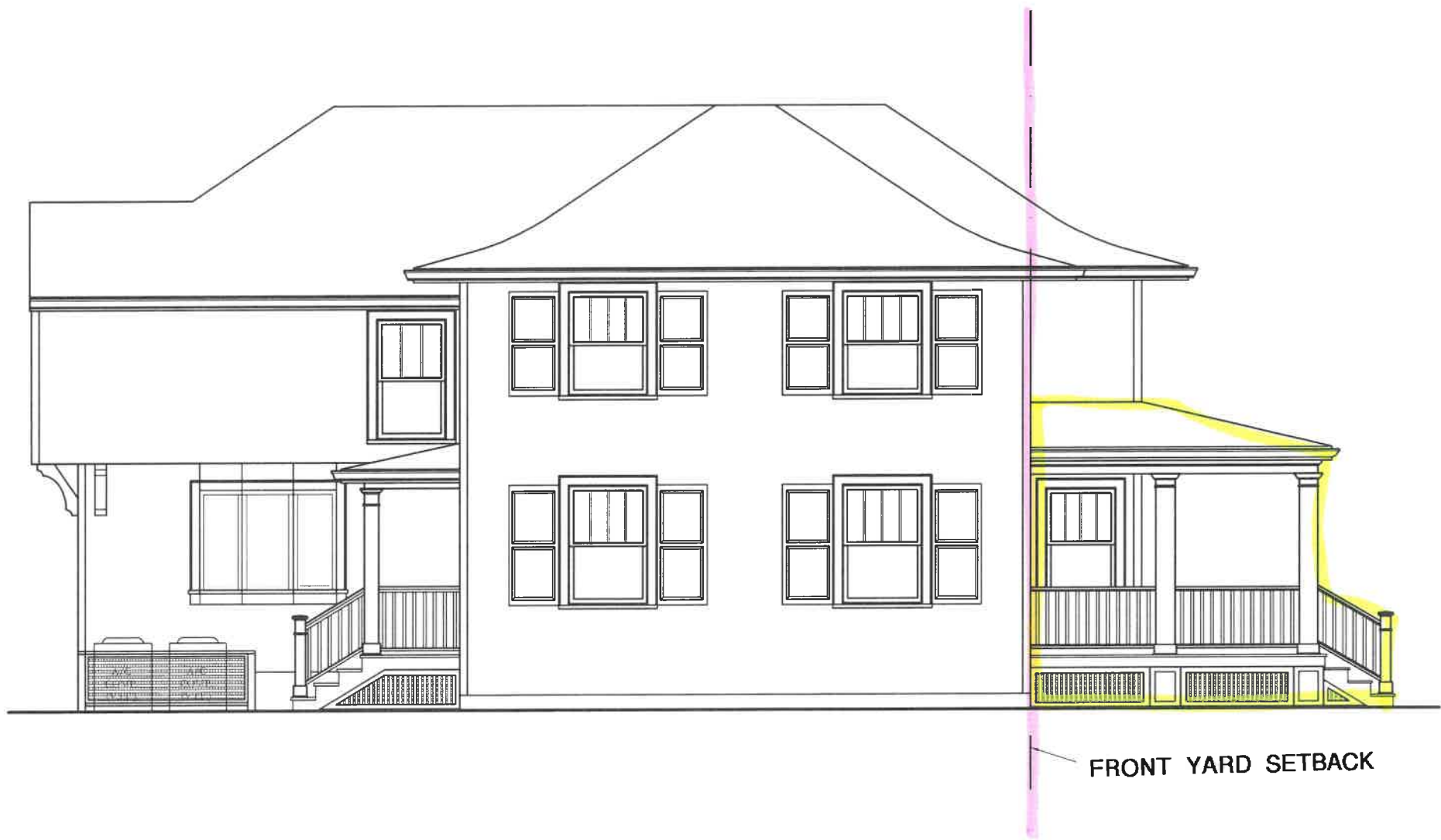
PROPOSED EAST ELEVATION
