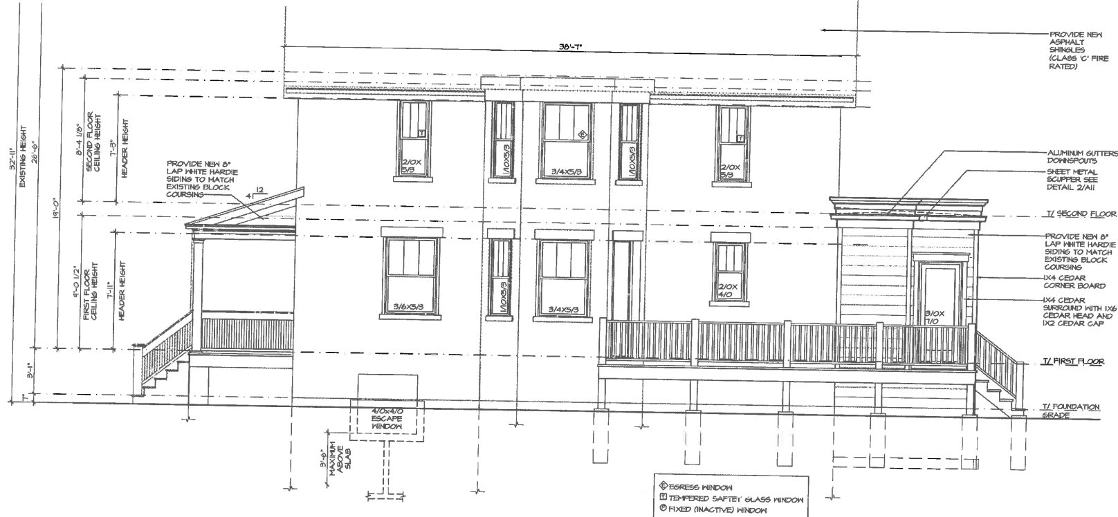
2 RIGHT ELEVATION (EAST) A 08 PROPOSED SCALE: 1/4"=1'-0"
