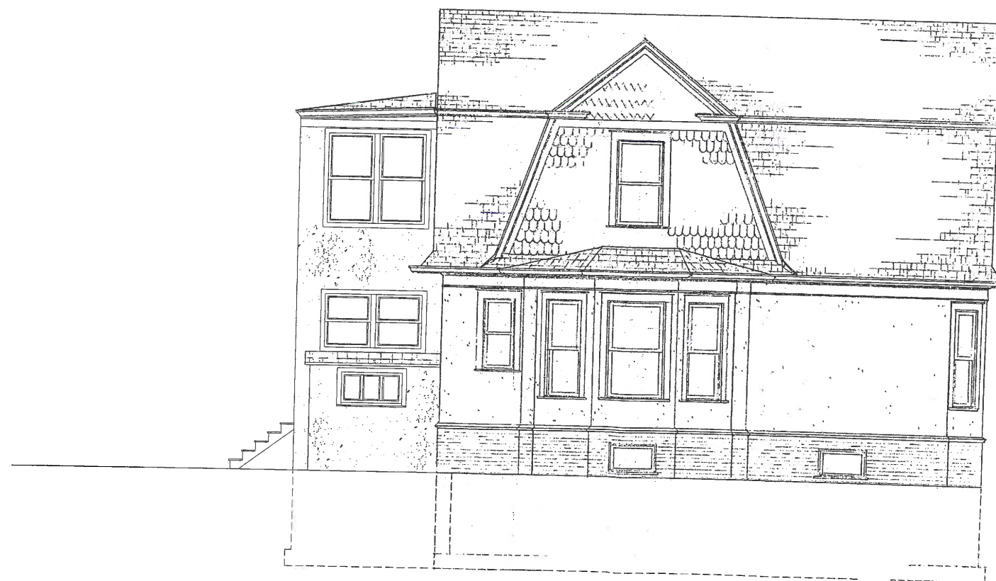
2 WEST ELEVATION - EXISTING SCALE: 1/4" = 1'-0"
