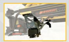
**Foot-end Hitch** Secures the foot end of the cot into the Power-LOAD system for transport.
