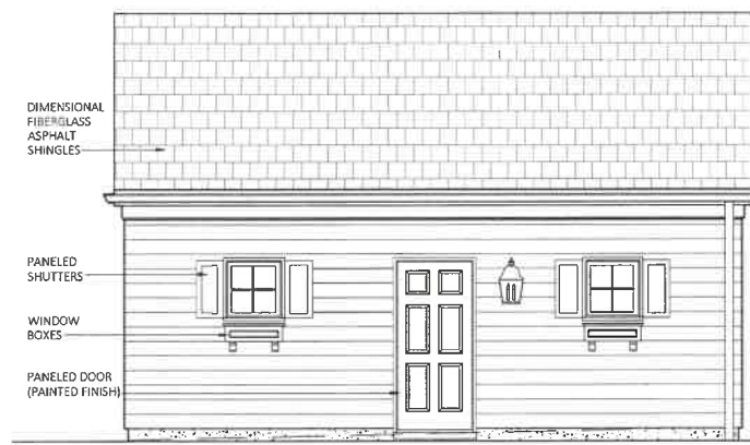
3 SOUTH ELEVATION Scale: 1/8"=1'-0"
