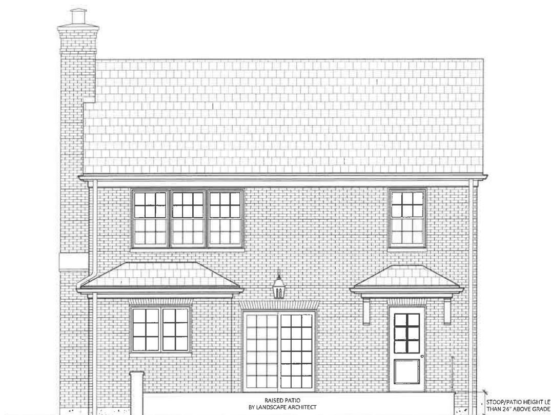
C REAR ELEVATION (East) Scale: 1/8"=1'-0"
