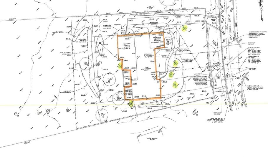
1. PROPOSED TOP OF NEW FOUNDATION AS NOTED ON PLANS, EXPOSED FOUNDATION SHALL BE MINIMUM OF 4" AND A MAXIMUM OF 8".
