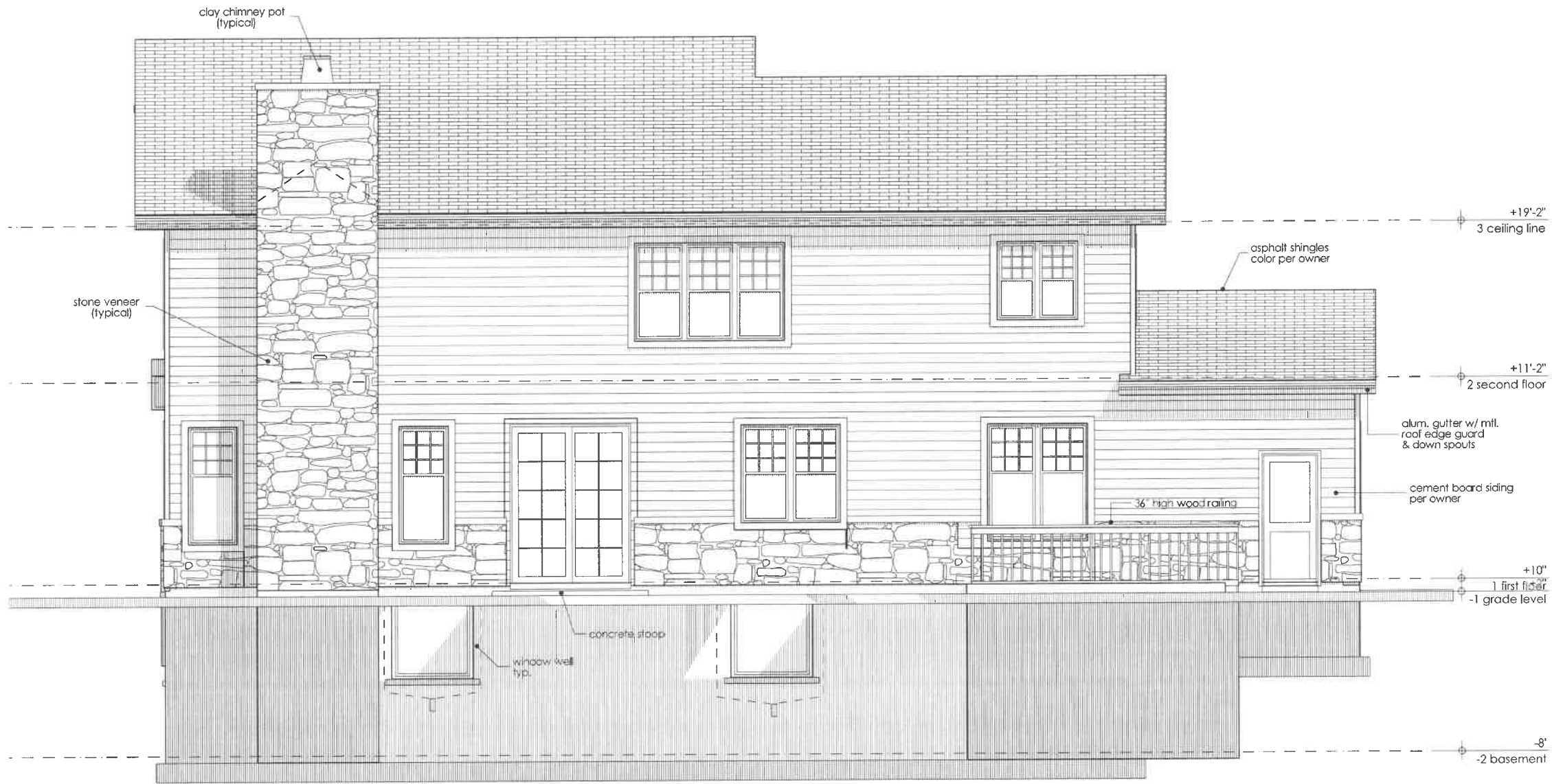
Rear Elevation SCALE: 1/4" = 1'-0"
