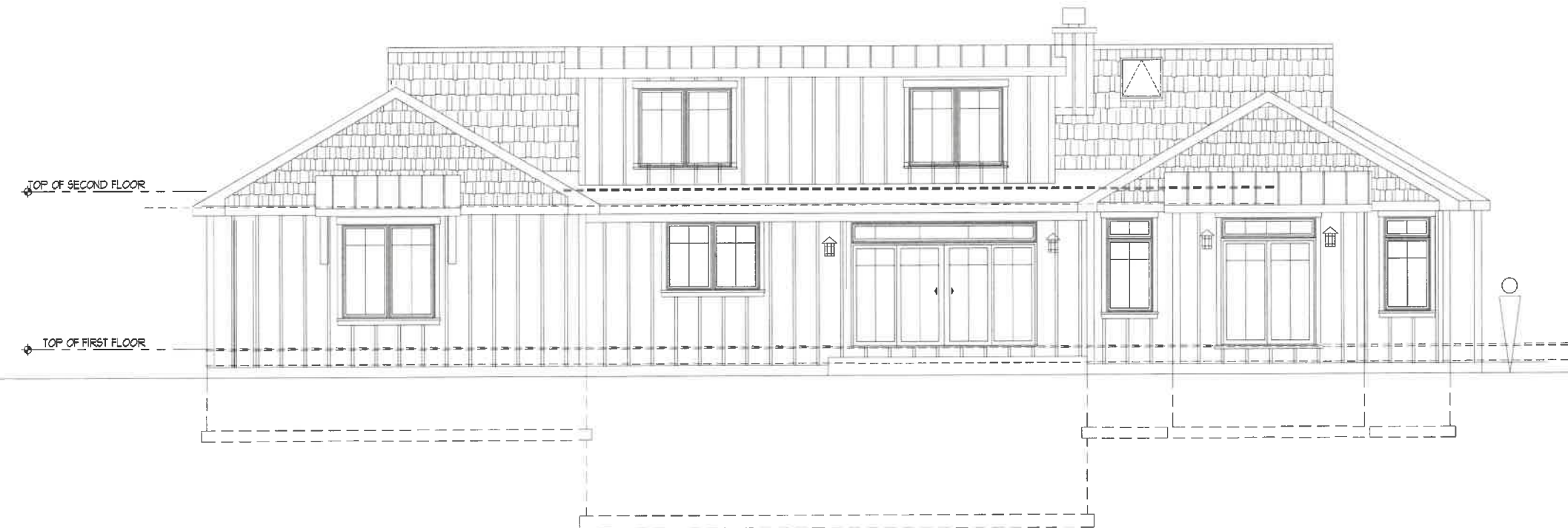
1 A-5 PROPOSED WEST ELEVATION SCALE: 1/4" = 1' - 0" BOARD AND BATTEN SIDING, ASPHALT MAIN ROOF W/ METAL ROOF ACCENTS
