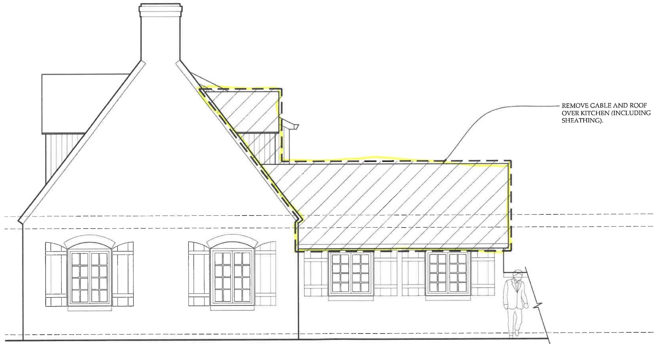
EXISTING SOUTH ELEVATION 1450 WEST OLD MILL ROAD
