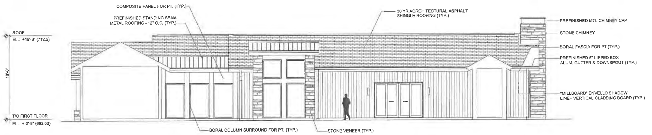
2 EXTERIOR ELEVATION - EAST 1/4" = 1'-0"
